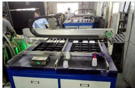
Battery Cover Gluing
